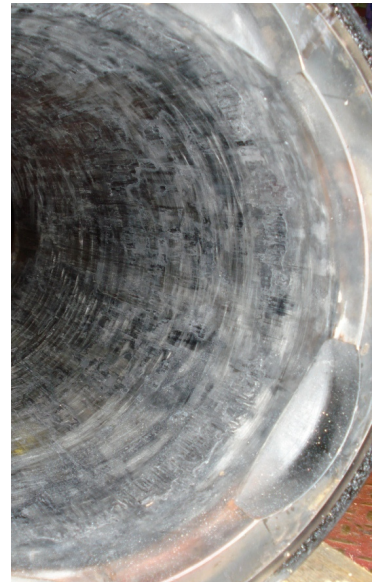
Damaged cylinder liner which can be a result of lack of lube oil
