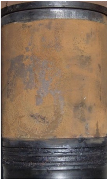
Cylinder liner damage due to poor cooling
