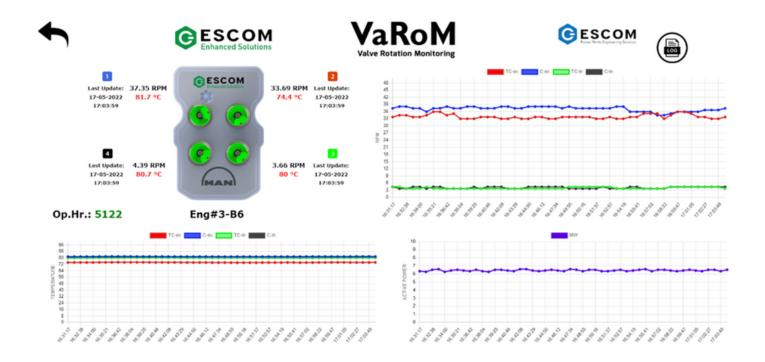
Easy-to-use SCADA application to visualize and analyze sensor data. Automatically collects BLE data sent from the sensor. Can store the data locally and visualize the data in HMI.
