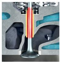
At a typical 750-RPM engine, each inlet/exhaust valve opens and closes 375 times a minute, each valve rotates app. 5/30 rev. per minute. and Inlet / Exhaust valves are designed to rotate, and this rotation is essential to valve longevity since it helps.
