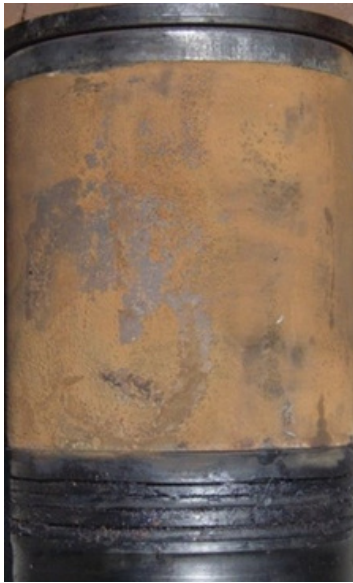
Cylinder liner damage due to poor cooling
